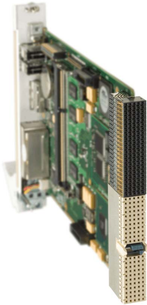
PC1-GROOVE • Backplane Connectors
