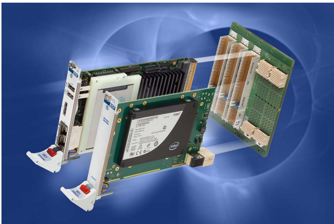
PC1-GROOVE as System Controller in a Hybrid System
