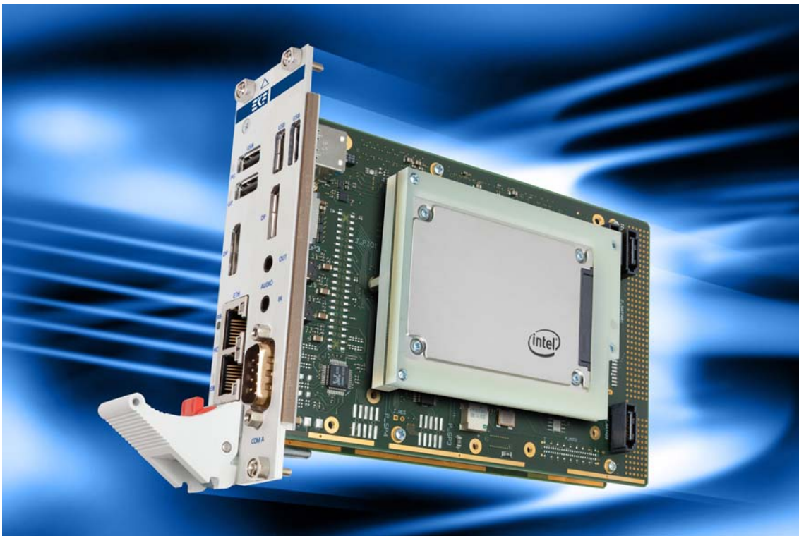
PC1-GROOVE w. PCS-BALLET Side Card & C42-SATA Mezzanine
