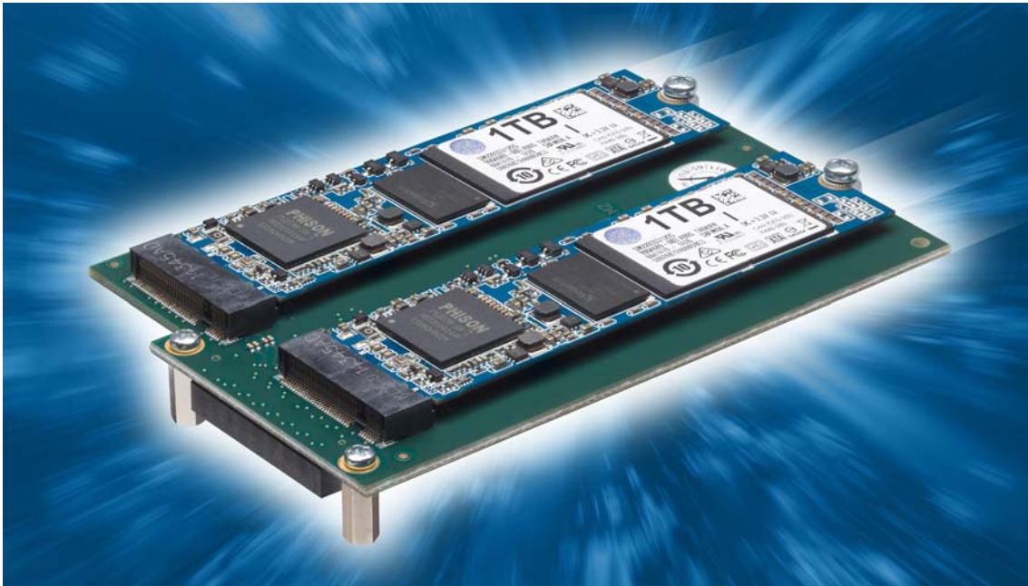
C48-M2 • Low Profile Storage Module 2 x M.2 SATA SSD
